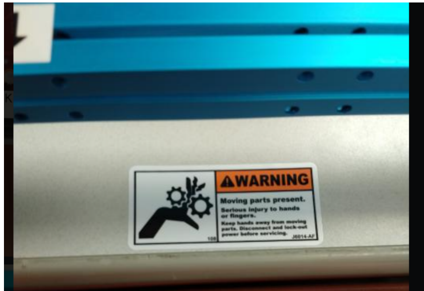
Figure 34: Pinch Hazard Label
